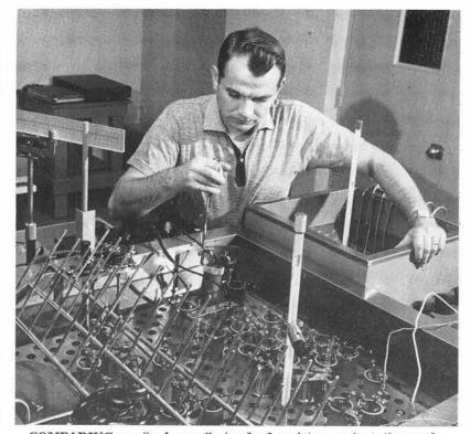
COMPARING an "unknown" standard resistor against the working standards of the Primary Lab, Don Eilar (2412-3) certifies the unknown and assigns it a value. This resistor is in turn used by a secondary lab as its reference standard. The resistors are maintained in an oil bath at 25° C. within plus or minus .02 of a degree.
